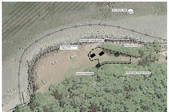
Design drawing shows the landing before restoration and new smaller area outlined with dashes and picnic tables
